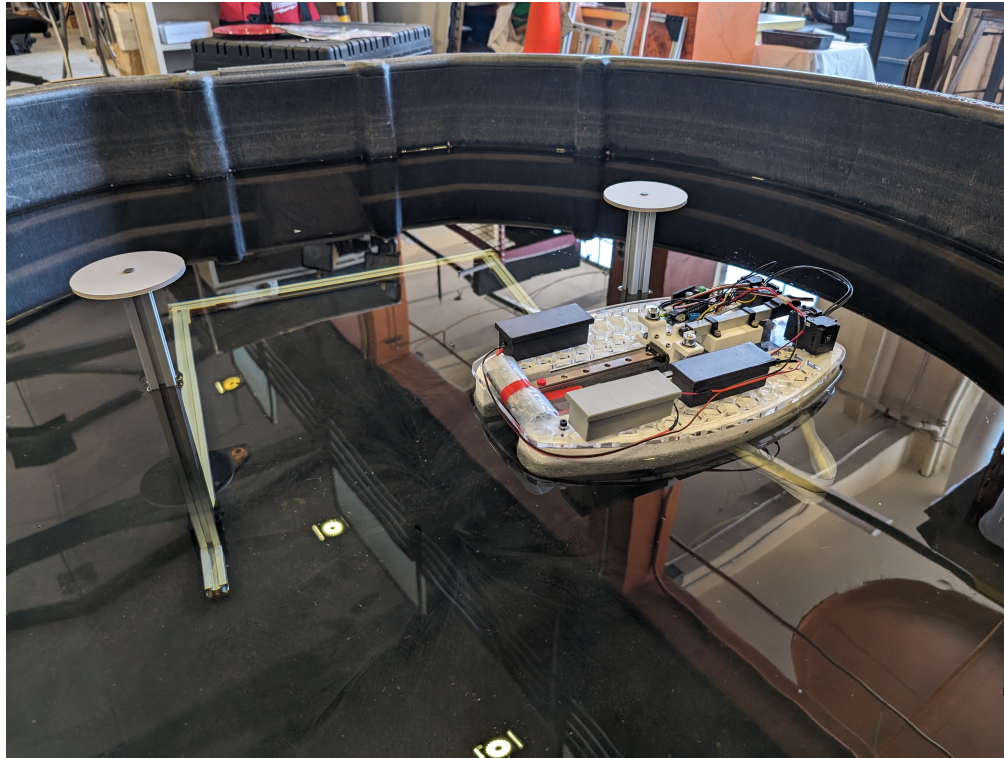
Figure 4.15: A side-view of the experimental test-tank for the figure-eight experiment. An aluminum frame was inserted into the test tank and topped with white visual markers to indicate the structure in the video.
