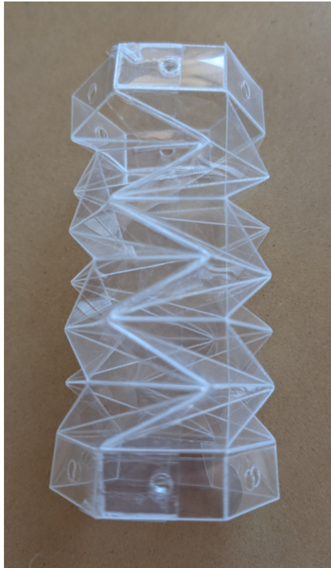
Figure 3.14: Photo of a folded and taped origami collapsible cylinder made from 3 collapsible antichiral Kresling-layer pairs. This is what the origami module looks like before it is bolted to the 3D printed endcaps using M3 bolts.
