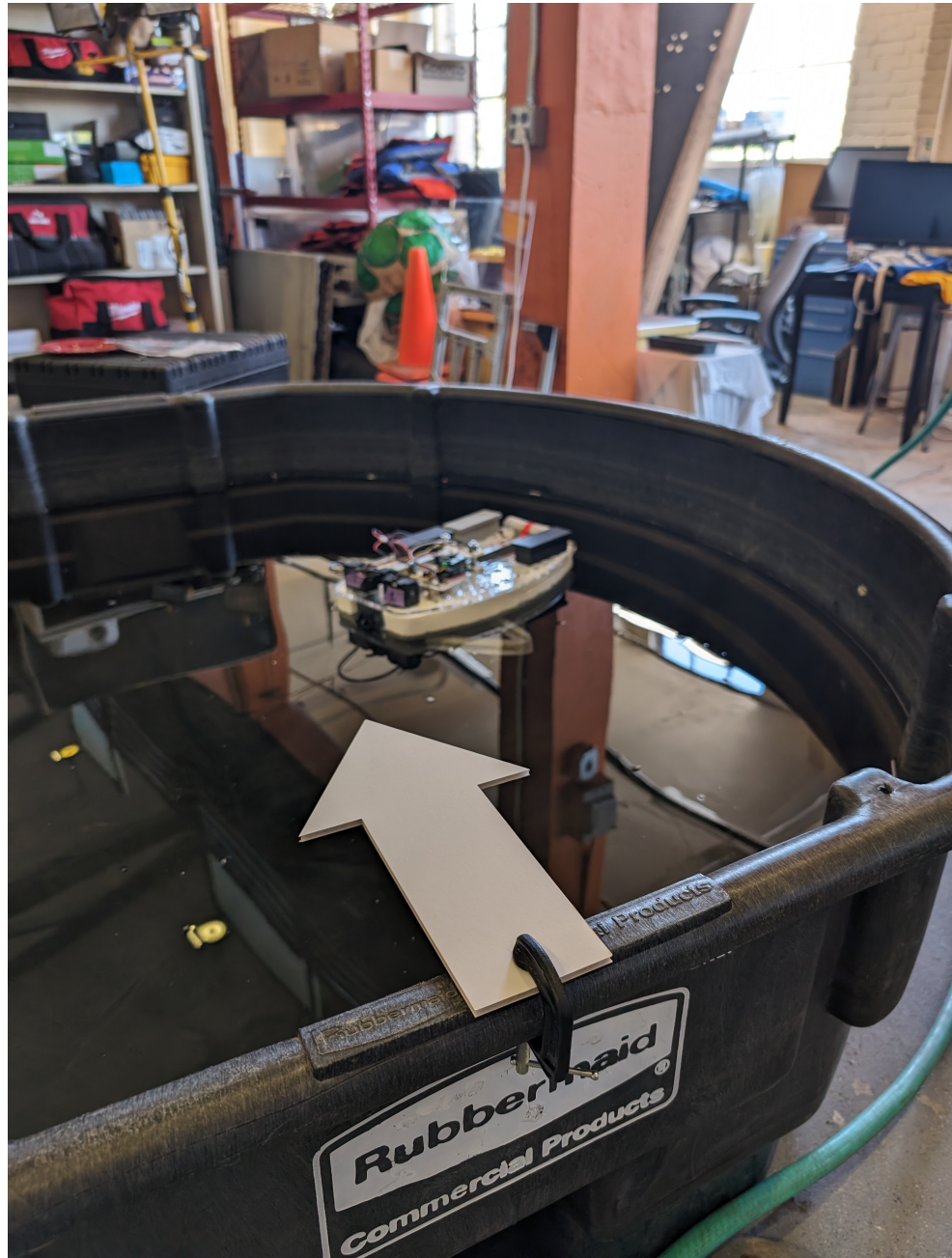
Figure 4.13: A side-view of the experimental test-tank for the waypoint navigation experiment. Two white posterboard arrows were clamped to the edges of the test tank, providing position and orientation waypoints to navigate between.
